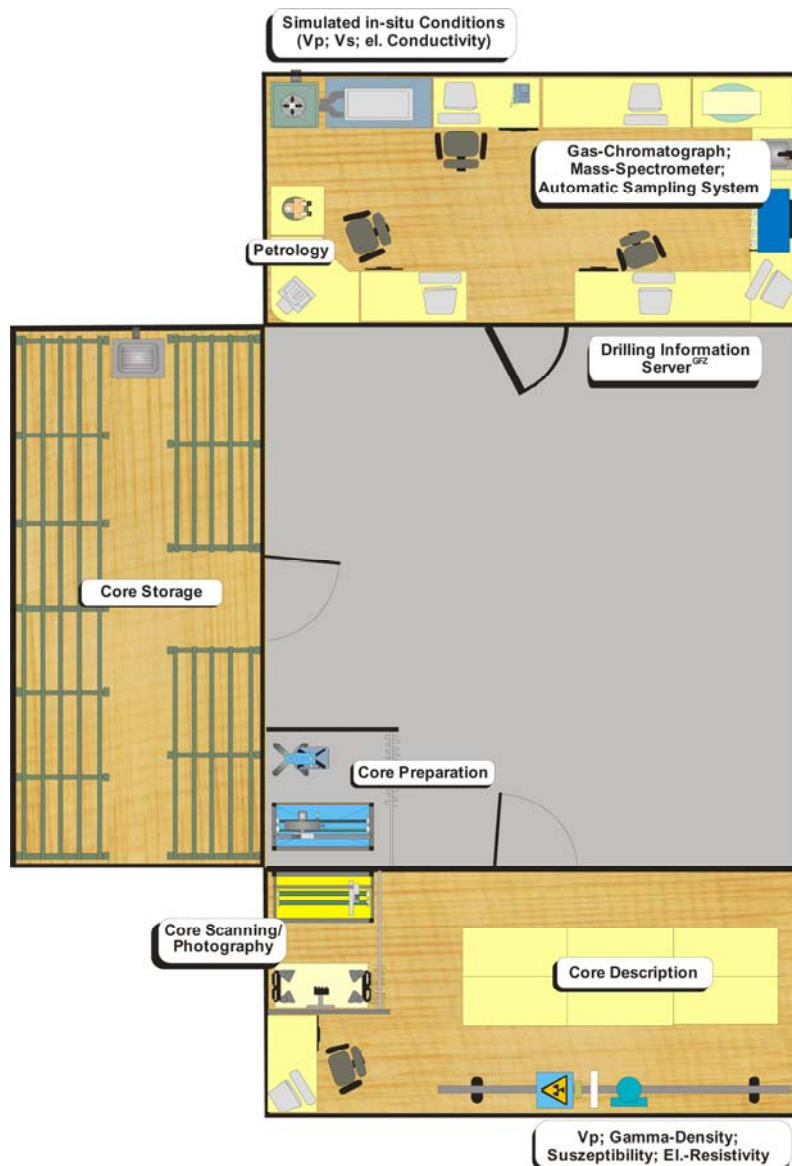
Fig. 7: Sketch and standard equipment for hard rock projects.
